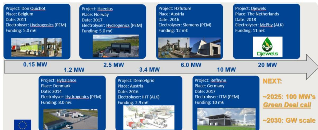
Figure 1: Overview of increased capacity of electrolyser for hydrogen production in the EU, funded by FCH JU.
