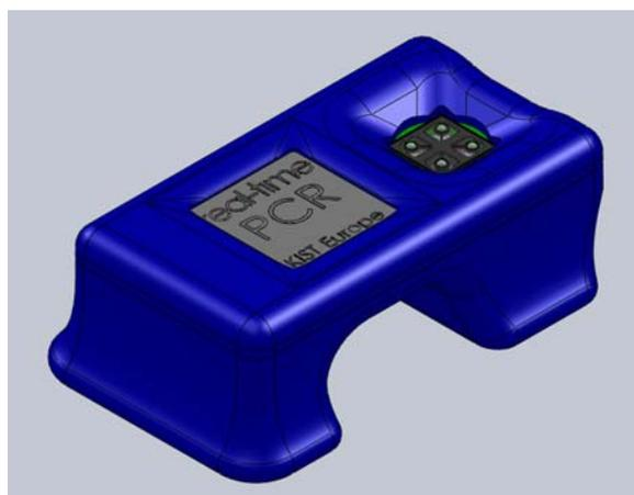
*Fig. 1: Computer added design (CAD) of complete PCR system with the housing.*
