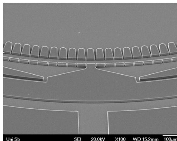
*Fig.2: SEM photo of the cell collector module. Small gaps between structures are 4.6 $\mu\text{m}$*
