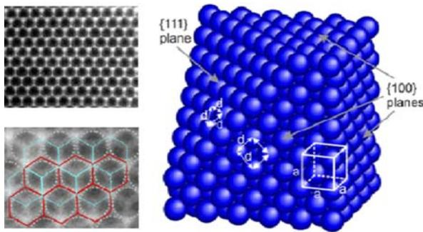
*Fig. 1: Self organized hexagonal oil nanodroplet droplet arrangements in a microchannel (left) and the schematic presentation of the face centered cubic (fcc) crystal structure (right).*
