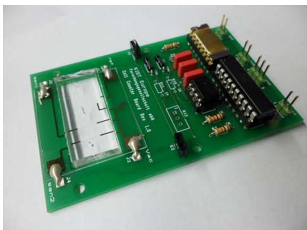
*Fig.1: Short facing cell counter chip and sensor electronics*
