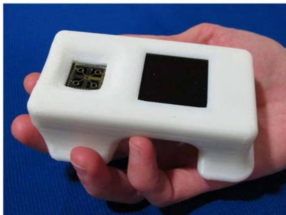
*Fig. 2: Assembled housing made by rapid prototyping technique with the electronics and display.*
