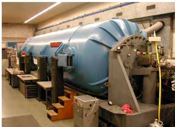
Figure 1: Van der Graaff generator ETH Zurich, capable of producing up to 6 million Volts (photograph from www.ams.ethz.ch ).
