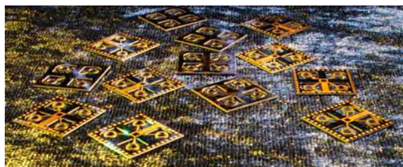
Figure 1: Micromachined silicon chips each with four integrated heaters and sensors
