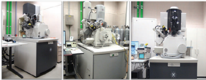
FIB equipment (FIB models: Nova600, Quanta3D, Helios)
