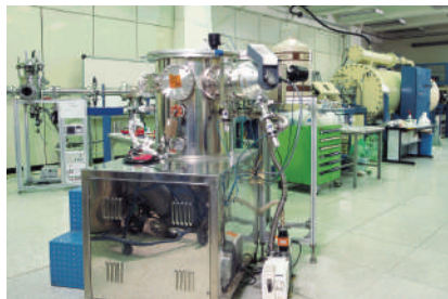
RBS instrument for the nano-analysis of material surface (Model: NEC 6SDH2)
