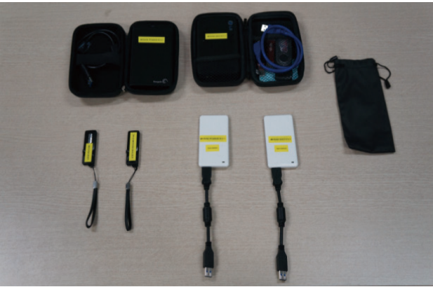
Figure 16. The KIST HPC management solution, USB flash drive type (64GB) and USB SSD type (128/256GB).
