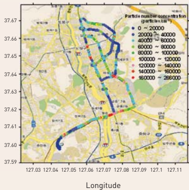
FIGURE 6. Spatial distribution of number concentration of particles larger than 5 nm measured with a mobile laboratory in Nowon-gu, Seoul, on October 5, 2010. [9]
