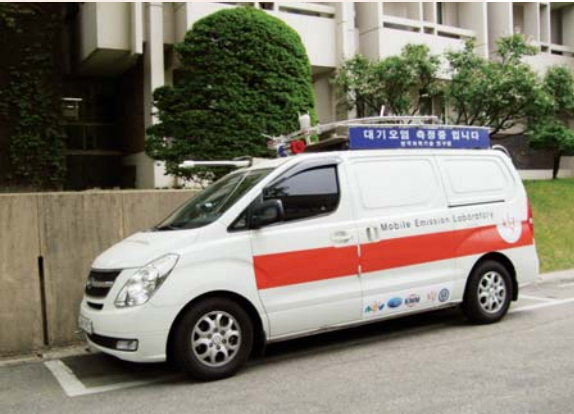
FIGURE 5. Multi-functional mobile laboratory for detailed monitoring of traffic-related air pollution.
