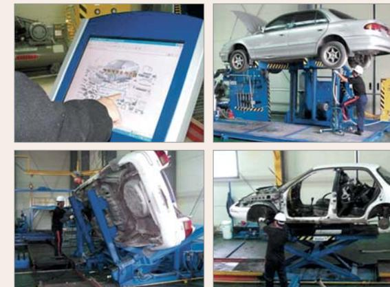
FIGURE 5. Construction and operation of dismantling system in pilot plant
