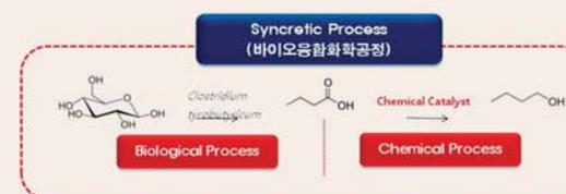
FIGURE 1. The syncretic process for butanol production
