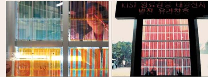
**FIGURE 5.** a) Colorful dye-sensitized solar cell; b) solar-powered window installed at KIST Kanneung branch.
